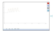
It is required to do minimum 5 complete pump cycles. The pump cycle speed should be approximately 30/minute for a 3 liter syringe and 60/min for a 1 liter syringe. The program stops automatically a few seconds after stopping pumping.
